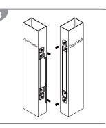
Tighten the fixing lugs with screws.
