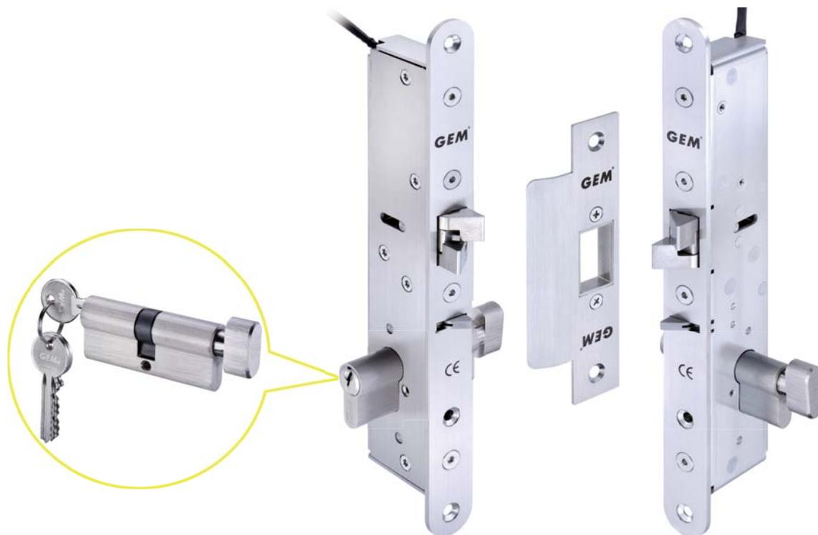
The ML-605M electric lock is a high performance lock designed for single action swing doors. Featuring a double action latchbolt and left/right side adjustable deadlatch tip, the ML-605M allows deadlocking automatically when the door is closed to be secured for ease of use and convenience. The ML-605M can be controlled by card readers/keypads and connected to automatic swing door operators for an integrated access control solution.
