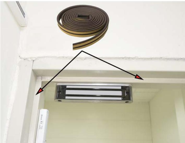
15. It is suggested to install the electromagnetic lock to prevent the door from being opened by force under wind load conditions or access control.
